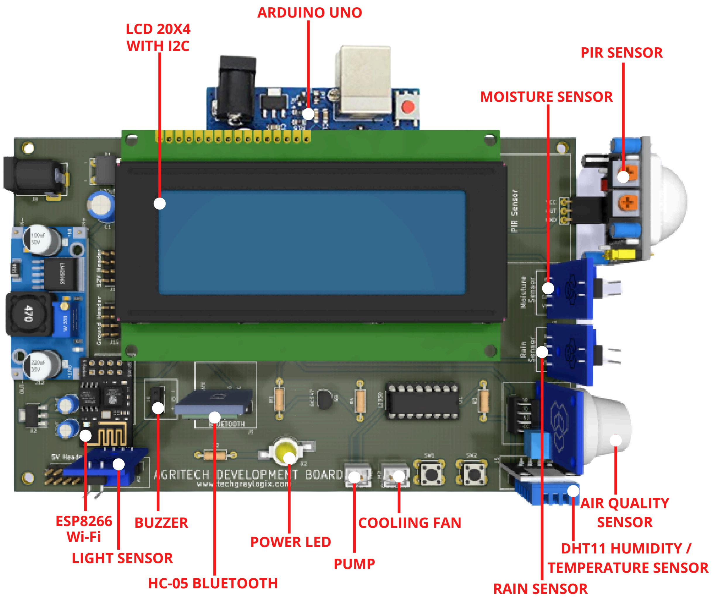
The development board has been specifically designed to fit variety of sensors, output devices and wireless modules. The aim is to decrease the amount of time required in rigging up the circuit and to maximize learning based on plug and play method.
